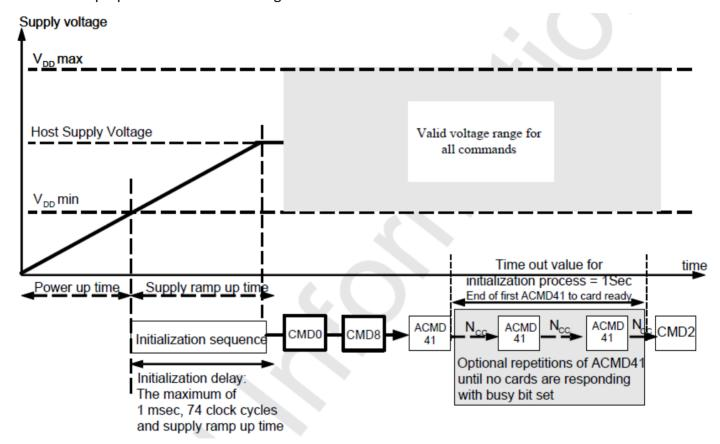
Power up time is defined as voltage rising time from 0 volt to VDD min and depends on application parameters such as the maximum number of SD Cards, the bus length and the characteristic of the power supply unit.
