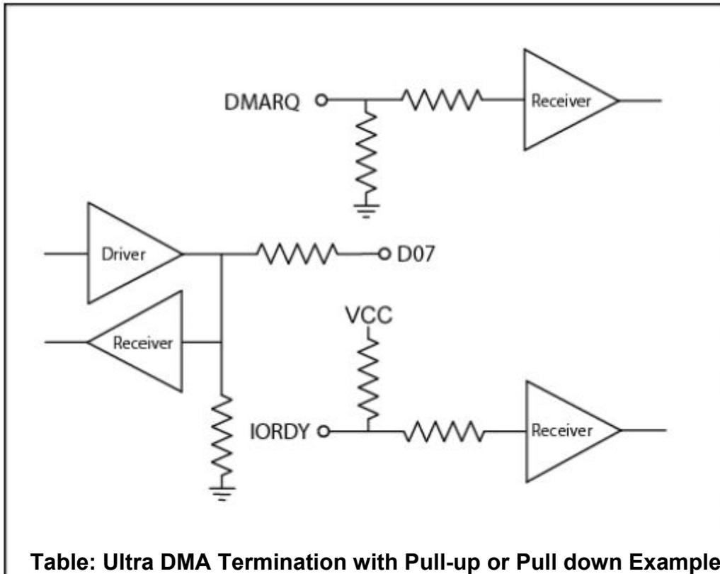
➤ **Printed Circuit Board (PCB) Trace Requirements for Ultra DMA**
